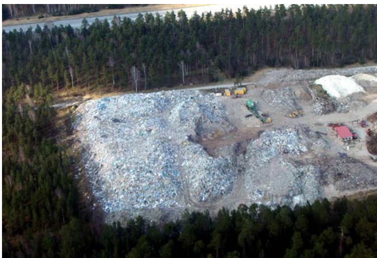
Figure 3. Typical intermediate deposit of recycling products in open space heap storage with 110,000 tons capacity.
