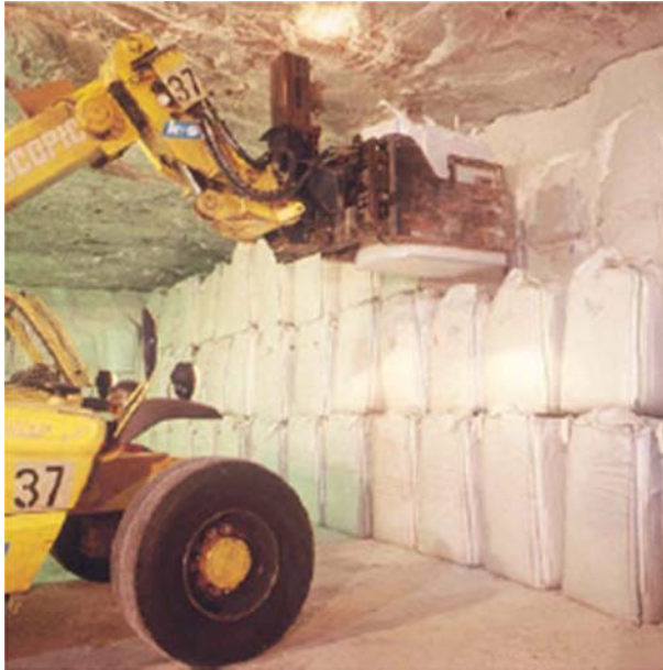
Figure 1. Example of underground storage of wastes (courtesy of BMG Engineering).
